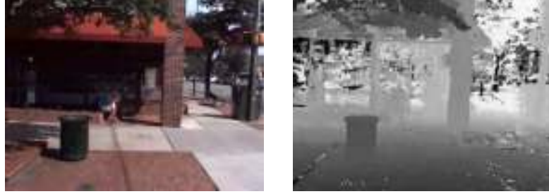
Figure 8.8: Left: Plane-sweeping stereo's reference image from an outdoor video sequence. Right: Depth map computed by plane-sweeping stereo using a total of eleven views.
