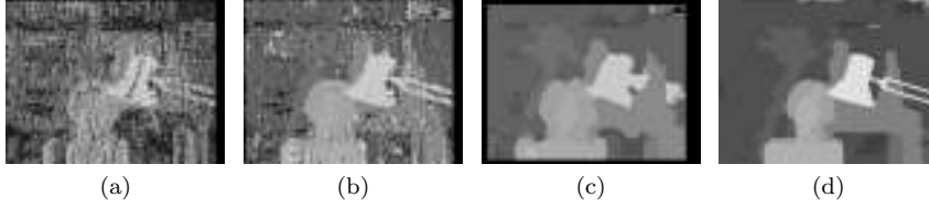
Figure 8.2: Different dissimilarity functions. (a) Pixel-wise matching solely based on color/intensity is highly ambiguous. (b) A 3 \times 3 correlation window is still noisy. (c) A 21 \times 21 correlation window results in edge fattening. (d) The cost filter method of [Hosni et al. 11b].
