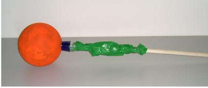
Figure 2: *The marker object that is tracked through the scene to establish 2D correspondences between camera frames.*
