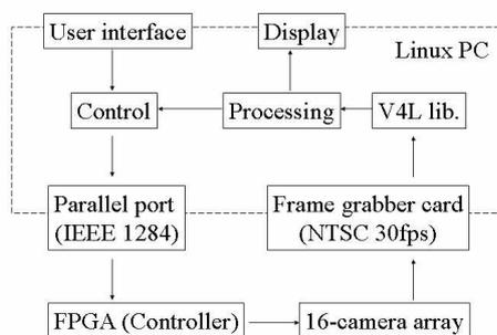
Figure 3: Video capture and control feedback loop
