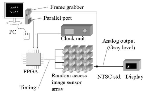
Figure 1: Block diagram of the imager array
