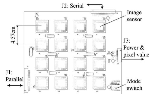
Figure 2: Layout of the sensor array
