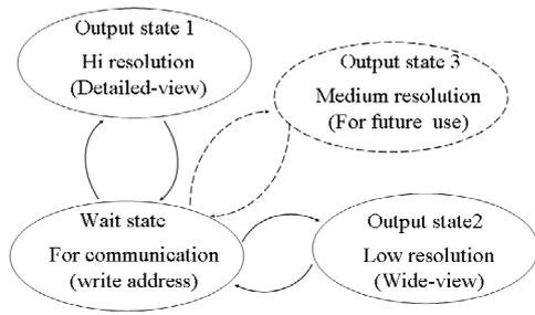
Figure 6: Operational states of CMOS imager
