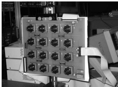
(a) Sensor array (FPGA on the backside)
