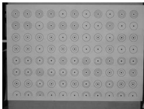
Figure 4: The calibration object
