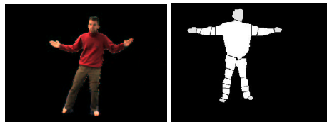
Figure 2: Video frame after background subtraction (l). GVD segmentation of silhouette in initialization position (r)
