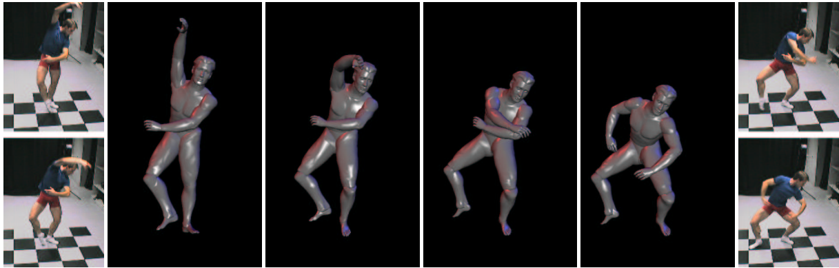
Figure 5: The four smaller images show subsequent video frames. Note the fast arm movement. In the four larger images, the corresponding poses of the body model are depicted as automatically estimated by the motion capture subsystem.
