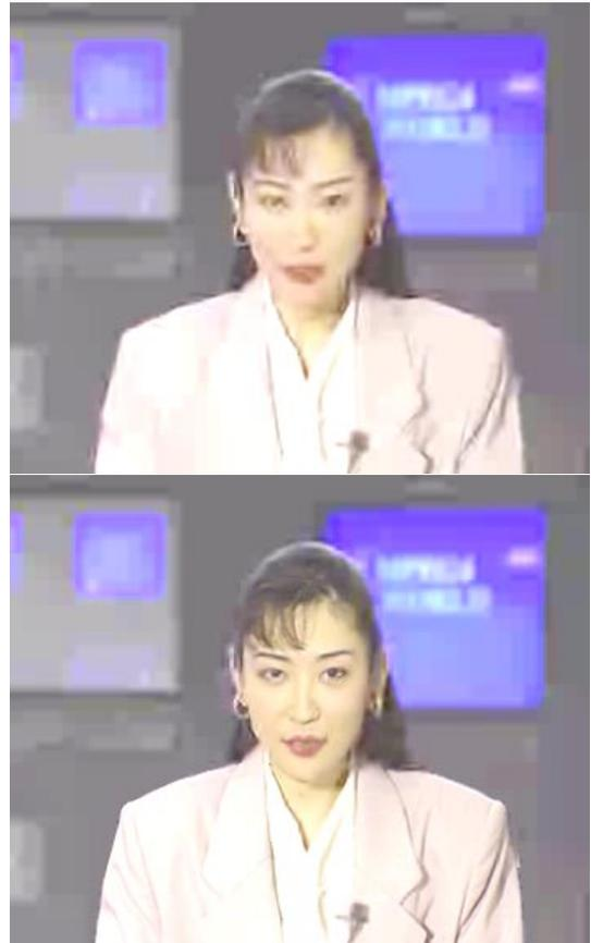
Figure 4: Frame 150 of the *Akiyo* sequence coded at the same bit-rate using the TMN-10 and the MAC, **upper image:** TMN-10 (31.08 dB PSNR, 720 bits), **lower image:** MAC (33.19 dB PSNR, 725 bits).
