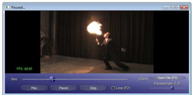
Fig. 3. The Graphical User Interface of our free viewpoint video player. In addition to traditional interface elements the user can control view direction (by dragging the mouse on the video) and playback rate (slider at bottom right).
