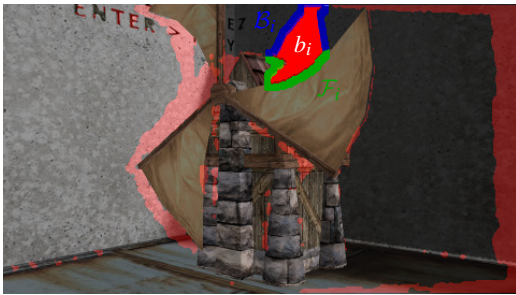
Figure 2: Flow repair: For each occluded blob, we determine two boundary classes \mathcal{F}_j (green) and \mathcal{B}_j (blue) by clustering the flow values along the boundary of the occluded blob b_i (red). For each boundary class, color statistics are computed in Lab space and each pixel of the occluded blob is inpainted with flow values from the most similar boundary.
